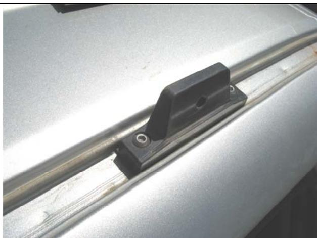
17. Place the rubber packer on the vehicle roof first and then the roof rack mounting block. Feed the M6 x 30 button head bolts through the vehicle roof.
