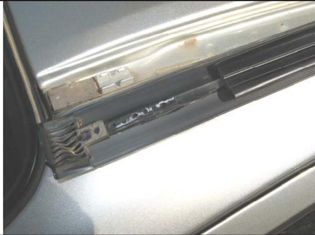
8. Remove the exterior roof trim from both sides of the vehicle. Take care not to bend the trim, as it will be reused.
