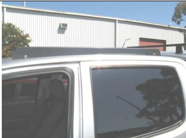
21. Fasten the mounting rails to the mounting blocks with M8 x 20mm button head screws, spring washers and flat washers and tighten.
