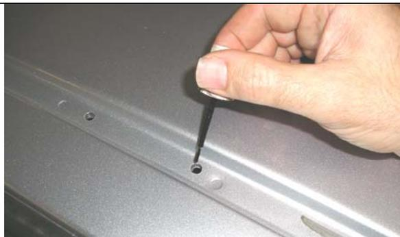
13. Remove all burrs and sharp edges from the newly drilled holes.
