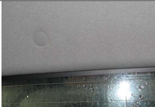
2. Remove the plugs located around the periphery of the ceiling. They are located at the front at the driver's side, the rear of the ceiling at the right and left hand sides of the vehicle and above the rear windscreen.
