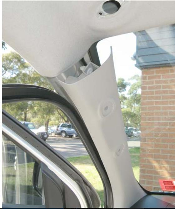
6. Remove the plastic trim from the front, middle and rear pillars on each side of the vehicle. They can simply be pulled away to be released from their mounting clips.
