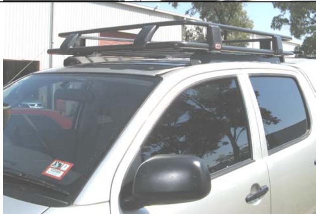
22. With the assistance of another person, lift the roof rack onto the vehicle and position evenly.
