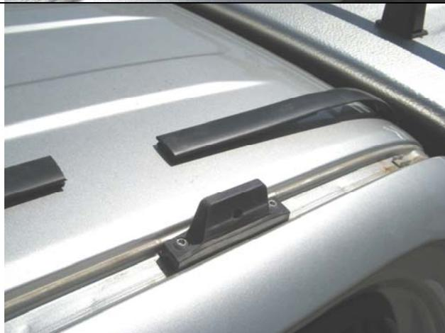
19. Cut the roof trim that was removed earlier at step 8 to fit neatly around the roof rack mounting blocks. There will be six pieces in total for both sides of the roof.
