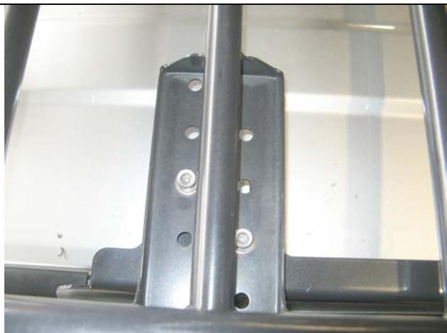
23. Fix the roof rack in place using eight M8 x 20mm socket head cap screws, M8 spring washers, M8 flat washers and four bolt plates. Tighten all bolts.
